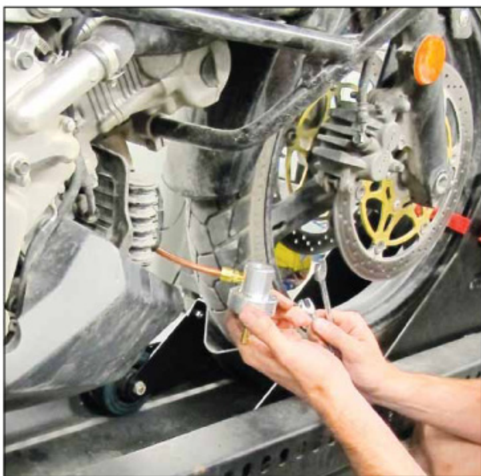
Dobeck oxygen sensor chamber is attached to the Bosch wide-band exhaust oxygen sensor probe.
