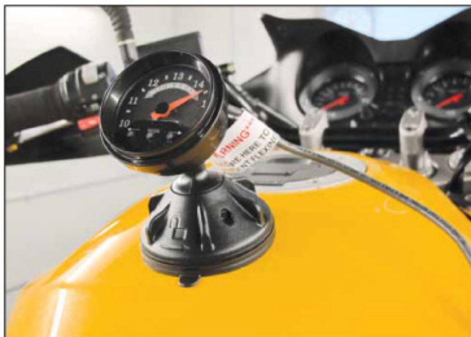
The Dobeck Performance SAFR unit is available for rent or purchase. See the air/fuel ratio, then decide if corrections are necessary.
